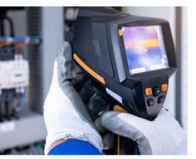
extremely beneficial in reducing electrical failures by identifying potentially dangerous conditions; such as loose or dirty connections, overloaded or imbalanced circuits, or improperly installed equipment. By measuring the heat imbalance relative to the environment and to surrounding equipment, abnormal or adverse conditions can be uncovered that if left unattended would worsen to the point of failure.
