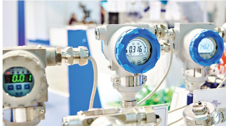
ASME B40.1 defines the accuracy grades of dial (analog) type gauges while ASME B40.7 defines the accuracy grades of digital gauges. For analog and digital pressure gauges the accuracy for grade 3A (code standard for test gauges) test gauges have an error of +/-0.25% span over the entire range.
