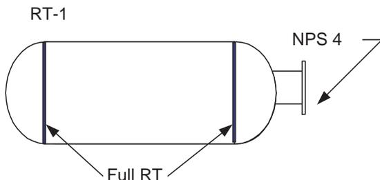
The two vessels are identical in thickness since in both cases a joint efficiency equal to 1.0 will be used in the shell hoop stress calculation and the head calculations. The shell axial stress calculations do not control the design even though the joint efficiency  $E$  is equal to 0.7 [assume Type 1 joints for the girth seams].
