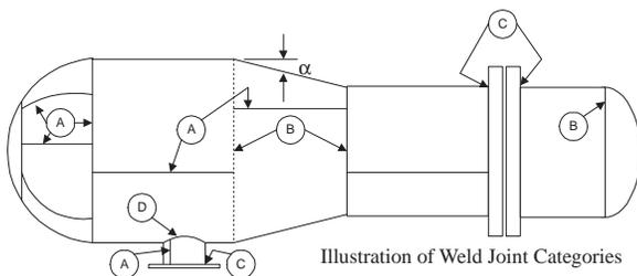
Category A: Longitudinal welded joints within main shells, heads, cones, flat plates, nozzles, and the attachment weld of a hemispherical head to a shell.
