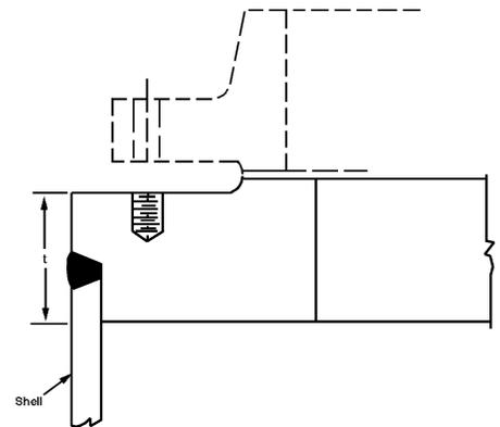
the presence of an inside fillet weld to reduce bending-related stress concentrations. Designs without the inside fillet weld are acceptable per 2-1(e) with acceptance of the Authorized Inspector. An upcoming revision in the '99 Addenda will provide an option for attaching a reverse flange with a full-penetration weld [see Fig. UW-13.2 sketch (d)] without the inside fillet weld.
