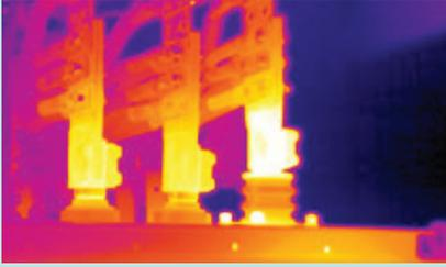
**Overheated transformer bushing**
