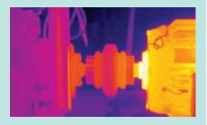
Under-lubricated motor bearing
